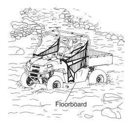
**NOTICE:** After running your vehicle in water, it's critical that you perform the services outlined in the Periodic Maintenance Chart beginning on page 59. Give special attention to engine oil, transmission oil, all gearcase fluids, and all grease fittings.
